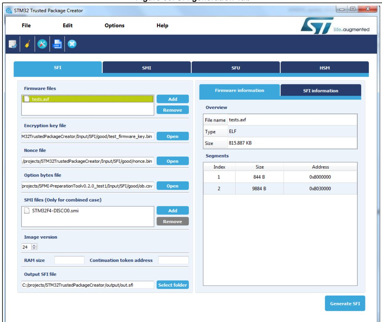
To generate an SFI image successfully from the supported input firmwares formats, the user must fill in the interface fields with valid values.
