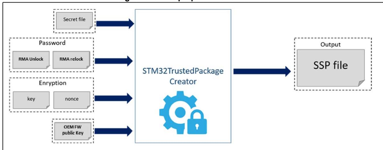
An SSP image must be created prior to SSP processing. The encrypted output file follows a specific layout that guarantees a secure transaction during transport and decryption based on the following inputs:
