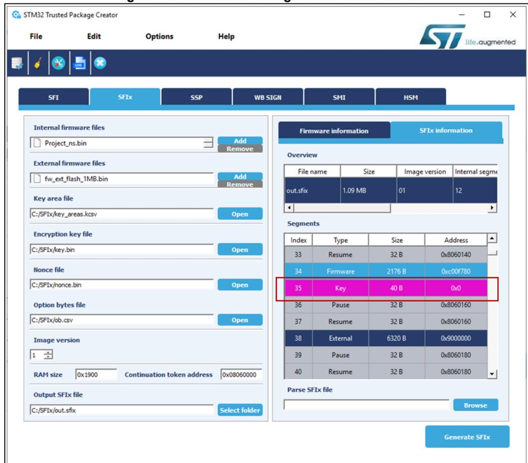
After the generation of the SFlx image in this use case the output file should contain 12 internal segments (F area), and 166 external segments (E area).
