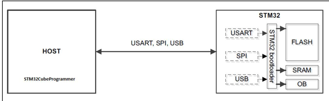
**Figure 45. Secure programming via STM32CubeProgrammer overview on STM32L4 devices**
