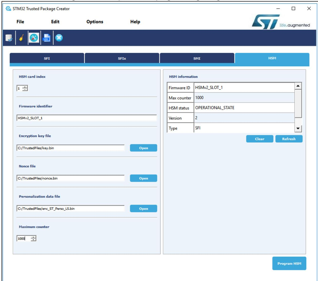
**Note:** When using HSM version 1, the “Personalization data file” field is ignored when programming starts. It is only used with HSM version 2.
