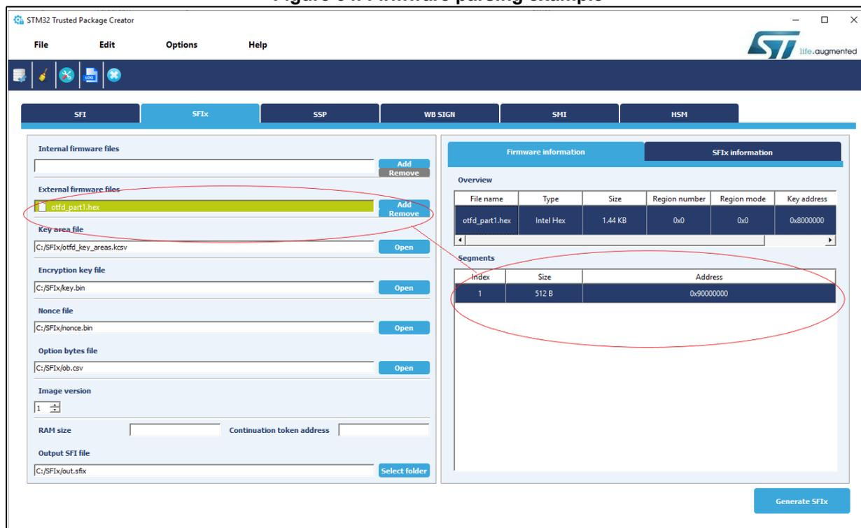
As is the case for the SFI use case, once all fields are filled in properly, the “Generate SFIx” button becomes enabled. The user can generate the SFIx file by a single click on it. If everything goes well, a message box indicating successful generation appears ([Figure 35: SFIx successful generation in GUI mode example](#)) and information about the generated SFIx file is displayed in the SFIx information section.
