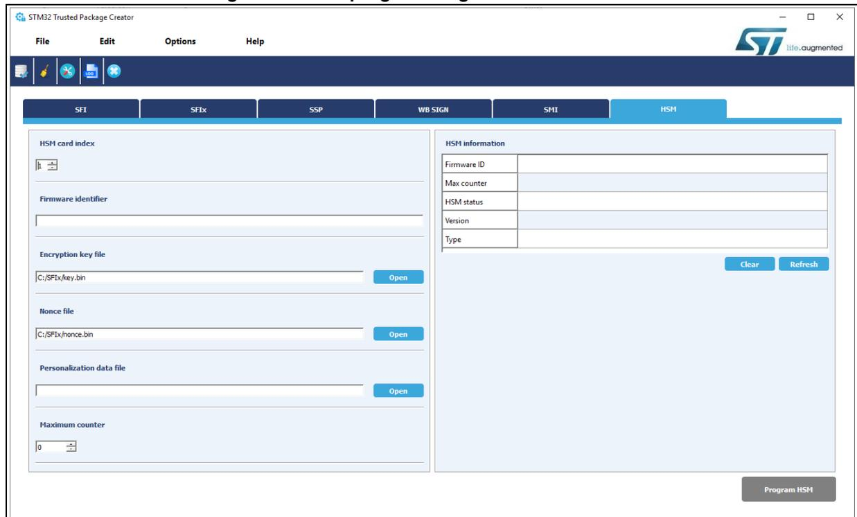
During SFI install, STM32CubeProgrammer communicates with the device to get the chip certificate, upload it into the HSM to request the license. Once the license is generated by the HSM, it gives it back to the STM32 device.
