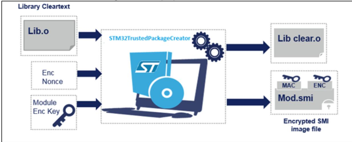
The SMI generation steps as currently implemented in the tool are described in the diagram below ([Figure 21](#)).
