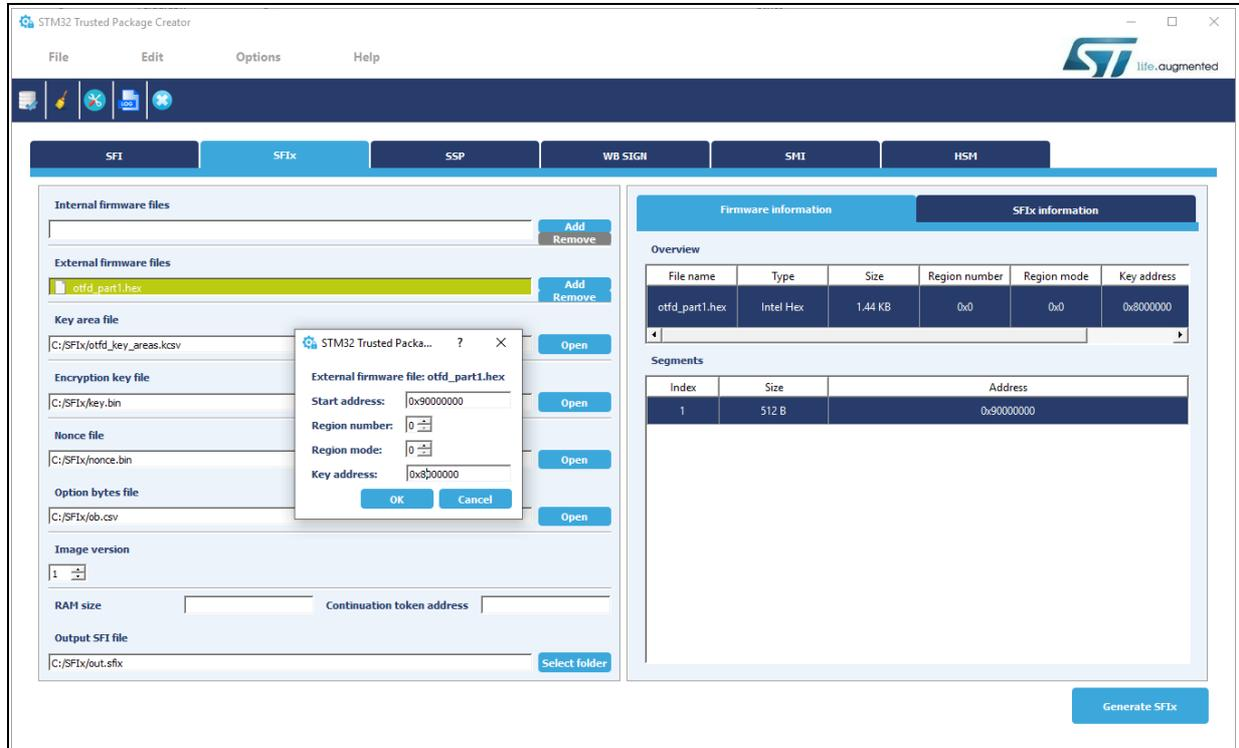
To generate an SFlx image successfully from the supported input firmware formats, the user must fill in the interface fields with valid values.
