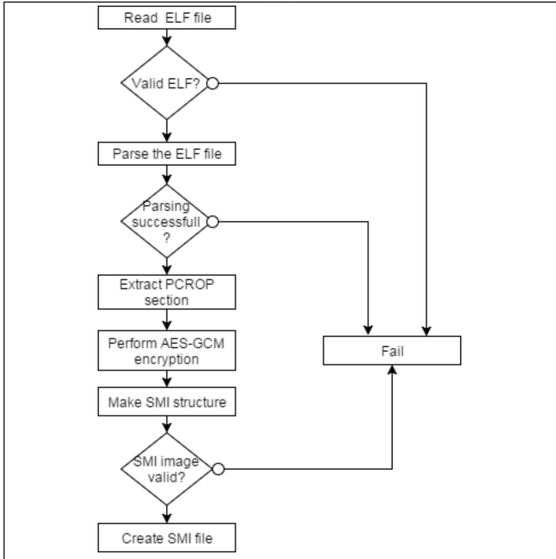
The AES-GCM encryption is performed using the following inputs:
