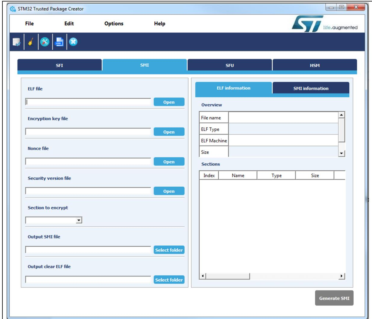
To generate an SMI image successfully from an Elf file, the user must fill in the interface fields with valid values.
