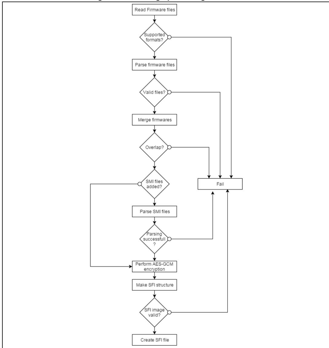
Before performing AES-GCM to encrypt an area, we calculate the Initialization Vector (IV) as:
