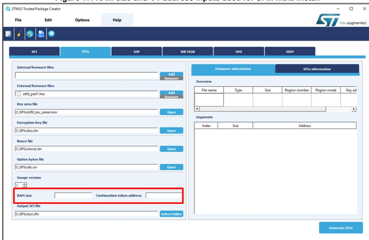
Note: To prepare an SFIx image from multiple firmware files, make sure that there is no overlap between their segments (Intern and extern), otherwise an error message appears as same as in the SFI use case.
