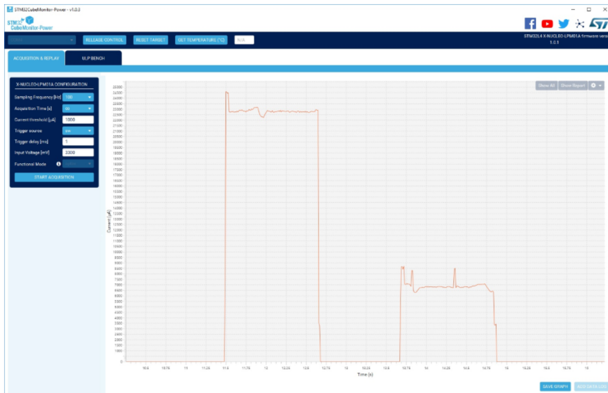
Figure 21. NUCLEO-WL55JC1 current consumption versus time
