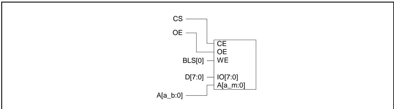
Figure 9: 8 Bit Bank External Memory Interface
