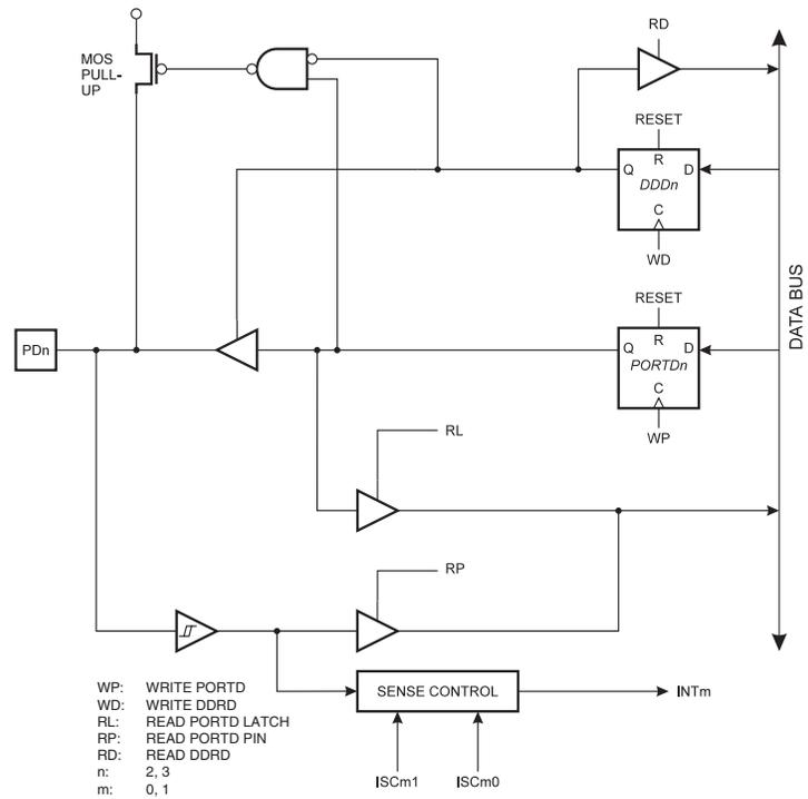
**Figure 67. Port D Schematic Diagram (Pin PD4)**
