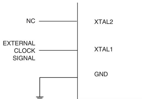
When this clock source is selected, start-up times are determined by the SUT Fuses as shown in Table 23.
