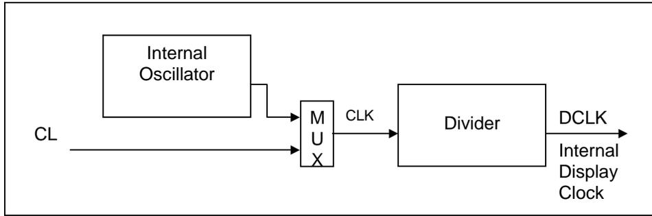
Figure 4 - Oscillator Circuit
