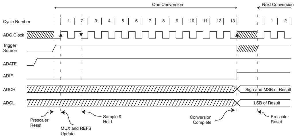
**Figure 119. ADC Timing Diagram, Free Running Conversion**
