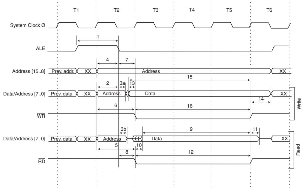
**Figure 86. External Memory Timing (SRWn1 = 1, SRWn0 = 1)<sup>(1)</sup>**
