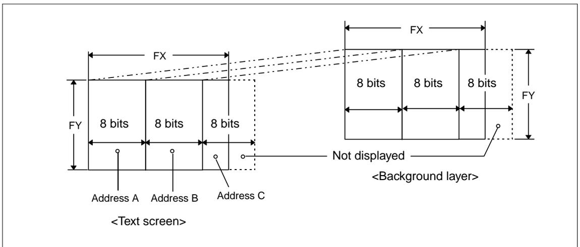
Figure 3-2 Typical relationship between FX/FY and display addresses
