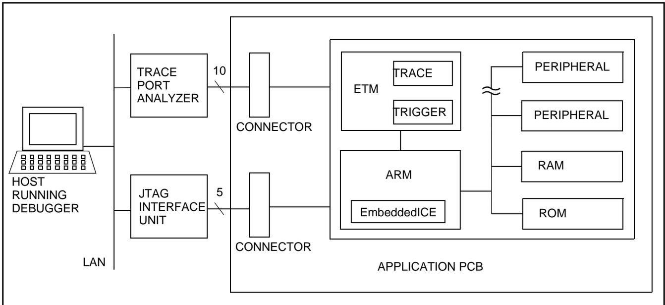
Figure 52: ETM Debug Environment Block Diagram
