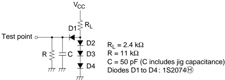
**HD61830B LCD Driver Interface ( $V_{CC} = 5V \pm 10\%$ ,  $GND = 0V$ ,  $T_a = -20$  to  $+75^\circ C$ )**
