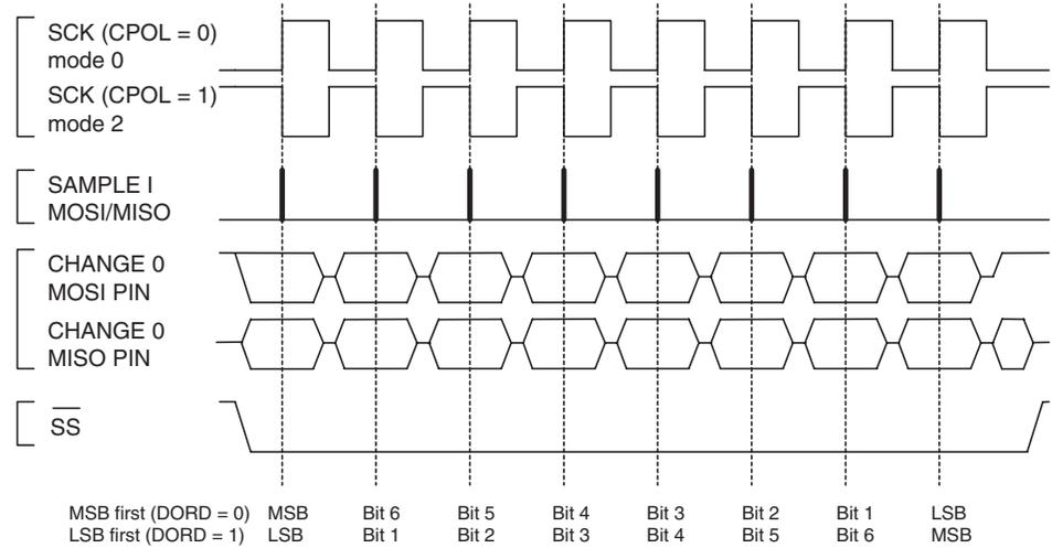
**Figure 81. SPI Transfer Format with CPHA = 1**
