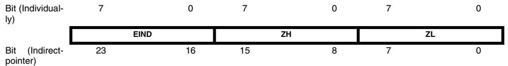
The actual number of bits is implementation dependent. Unused bits in an implementation will always read as zero. For compatibility with future devices, be sure to write these bits to zero.
