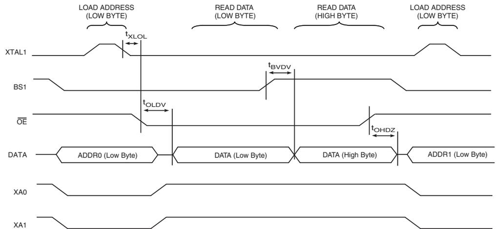
Note: 1. The timing requirements shown in Figure 144 (i.e.,  $t_{DVXH}$ ,  $t_{XHXL}$ , and  $t_{XLDX}$ ) also apply to reading operation.
