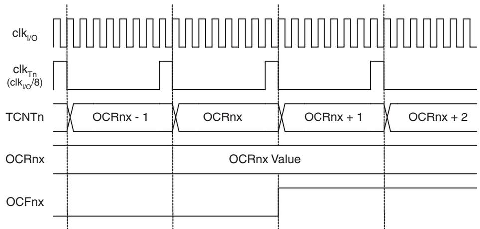
Figure 59 shows the count sequence close to TOP in various modes. When using phase and frequency correct PWM mode the OCRnx Register is updated at BOTTOM. The timing diagrams will be the same, but TOP should be replaced by BOTTOM, TOP-1 by
