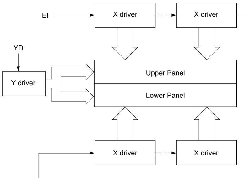
Figure 3. Above and below two-panel display
