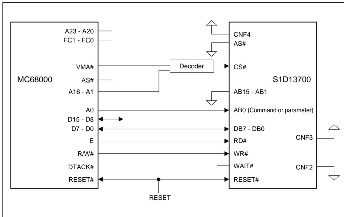
MC68000 System Block Diagram (direct)
