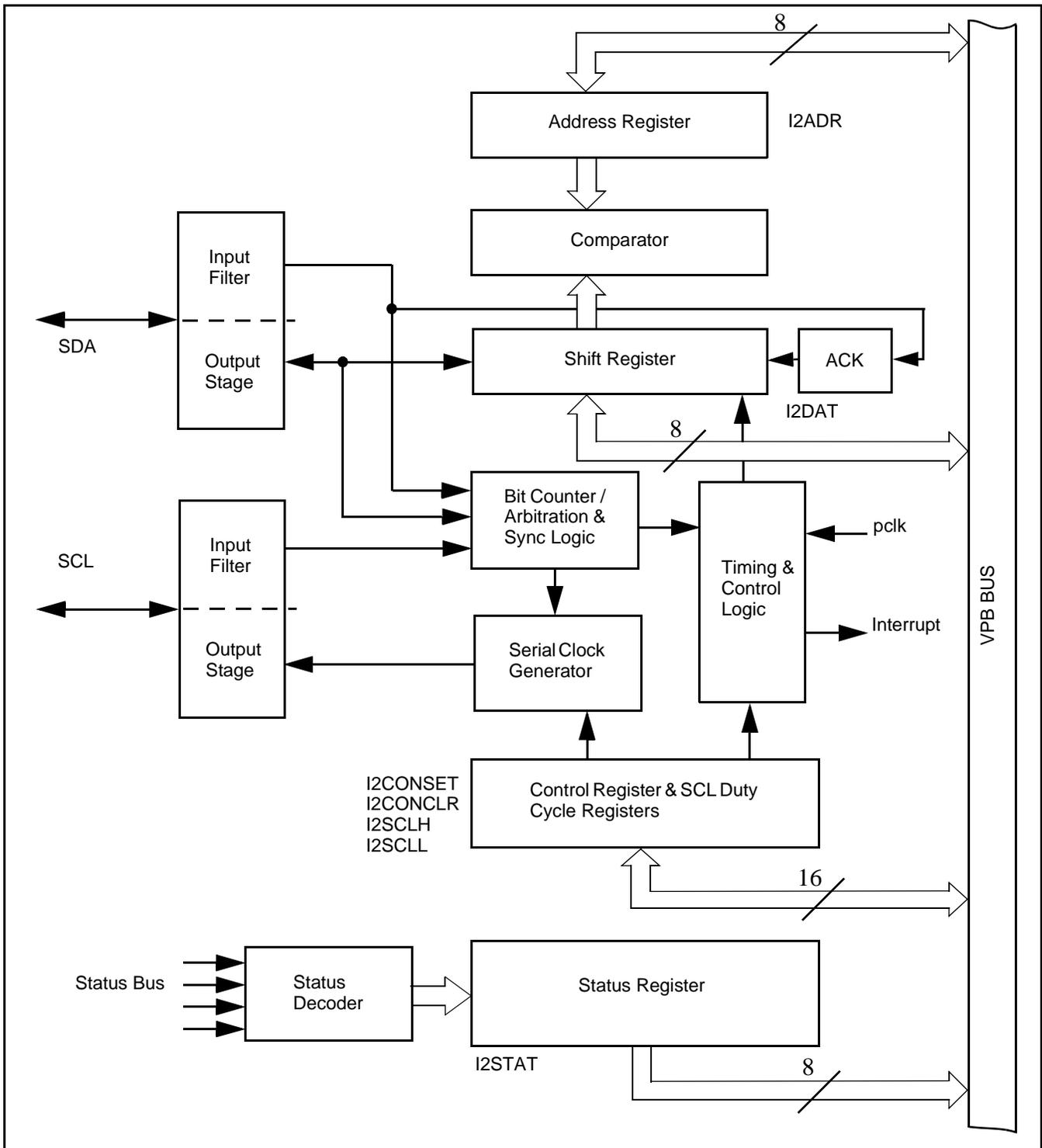
Figure 32: I<sup>2</sup>C Architecture
