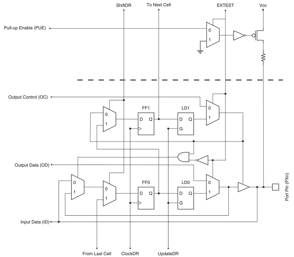
**Figure 133. General Port Pin Schematic Diagram**
