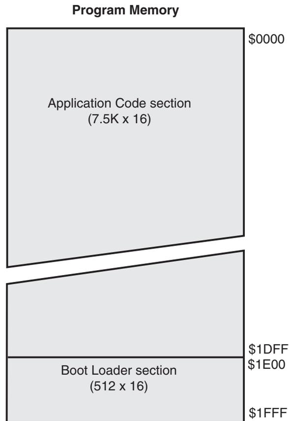
The Boot Loader program can use any available data interface and associated protocol, such as UART serial bus interface, to input or output program code and write (program) that code into the Flash memory or read the code from the Program memory.
