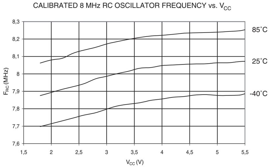
**Figure 204.** Calibrated 8 MHz RC Oscillator Frequency vs. Temperature
