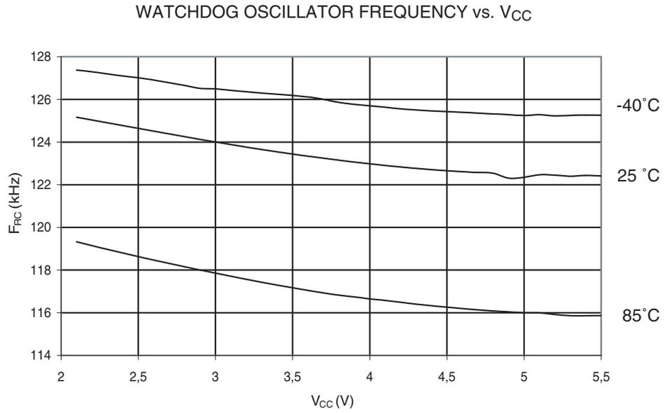
**Figure 202.** Watchdog Oscillator Frequency vs. Temperature
