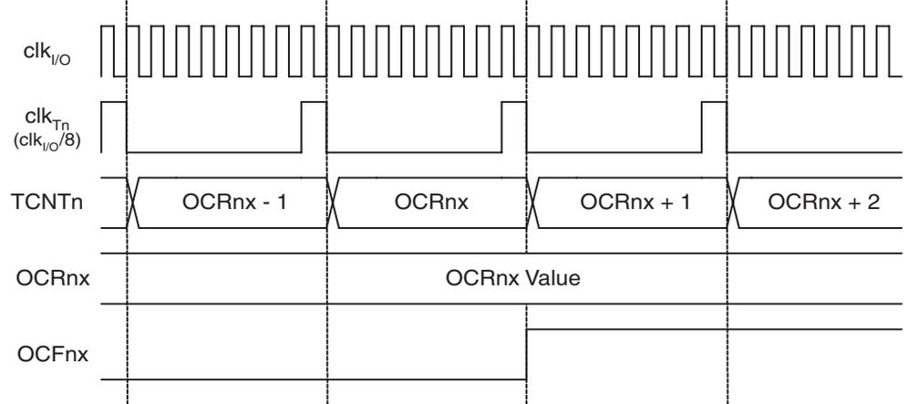
Figure 76 shows the setting of OCF2A and the clearing of TCNT2 in CTC mode.
