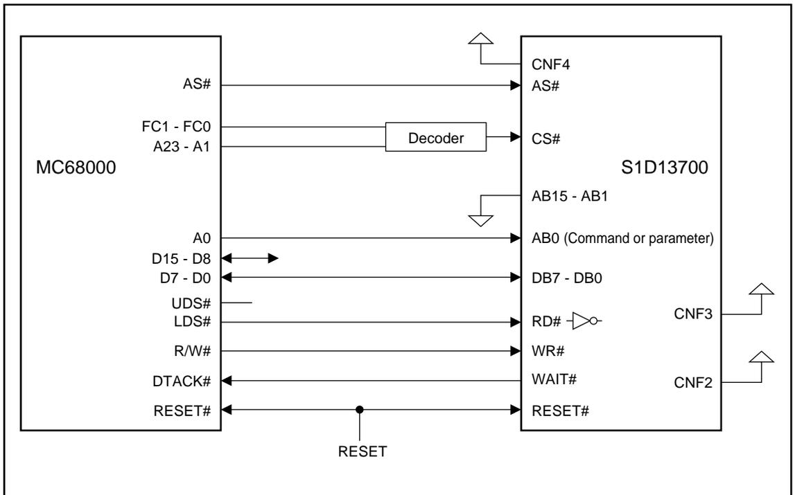
MC68000 System Block Diagram (direct)
