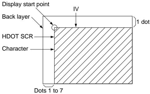
Figure 5. IV and HDOT SCR adjustment
