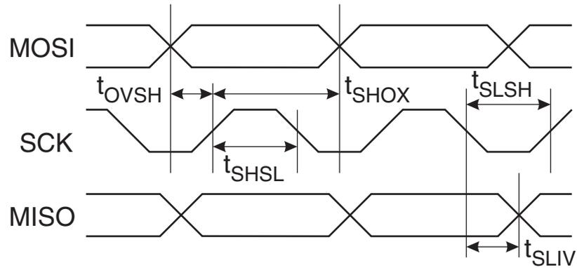
Table 49. Serial Programming Characteristics,  $T_A = -40^{\circ}\text{C}$  to  $85^{\circ}\text{C}$ ,  $V_{CC} = 2.7 - 5.5\text{V}$  (unless otherwise noted)
