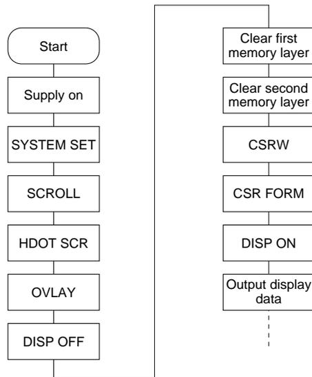
Figure 57. Initialization procedure
