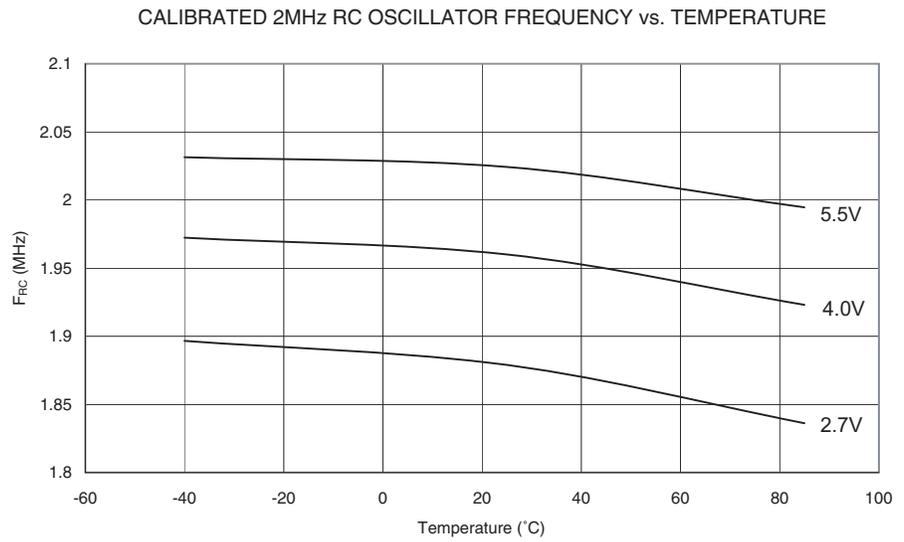
**Figure 201.** Calibrated 2 MHz RC Oscillator Frequency vs.  $V_{CC}$
