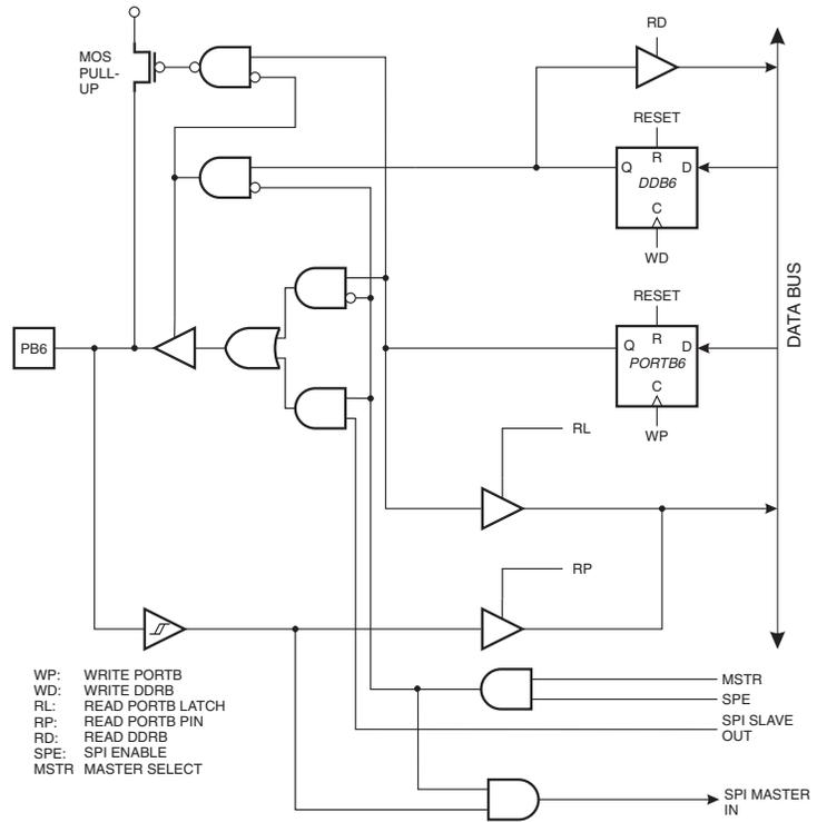
**Figure 62. Port B Schematic Diagram (Pin PB7)**
