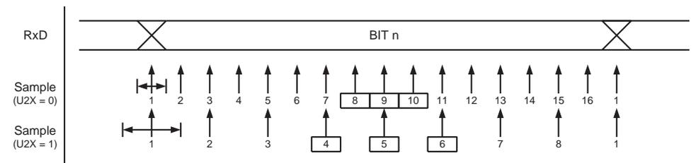
The decision of the logic level of the received bit is taken by doing a majority voting of the logic value to the three samples in the center of the received bit. The center samples
