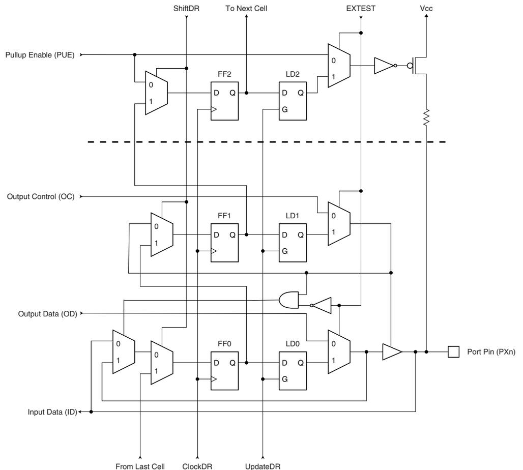
**Figure 117. General Port Pin Schematic Diagram<sup>(1)</sup>**
