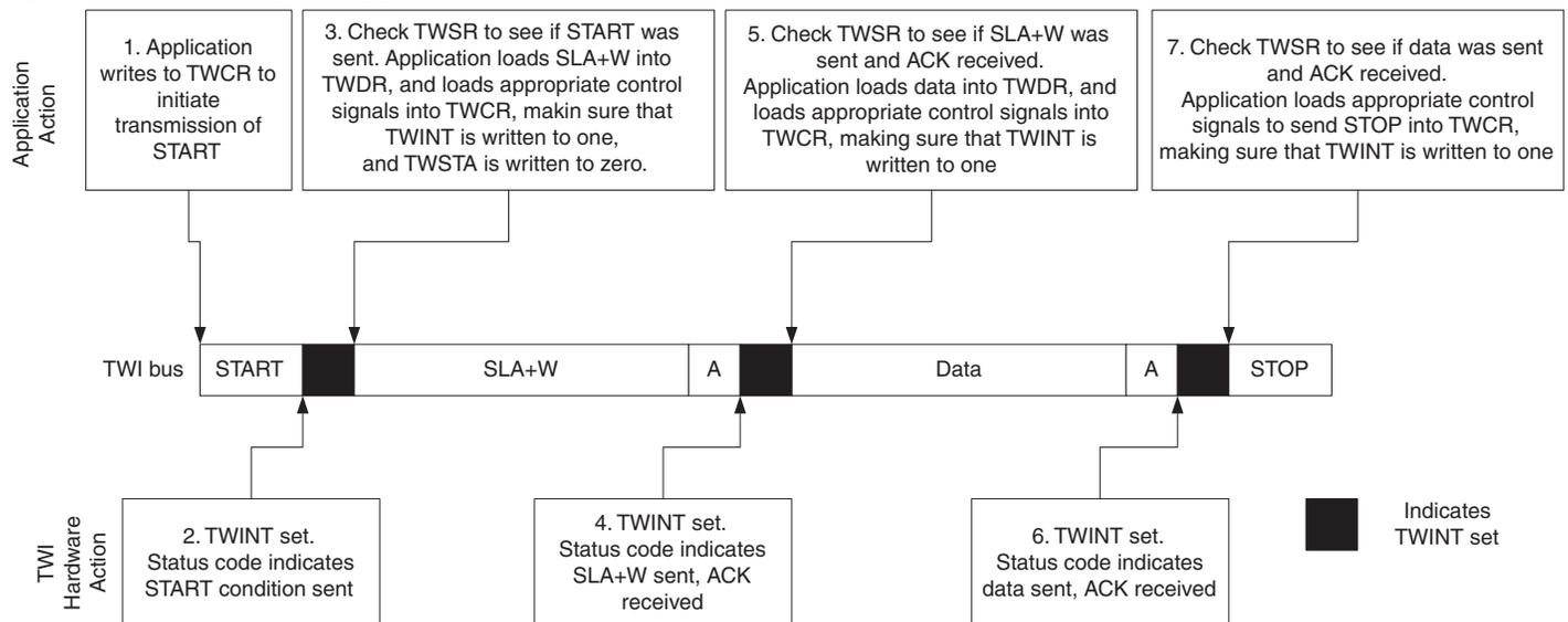
1. The first step in a TWI transmission is to transmit a START condition. This is done by writing a specific value into TWCR, instructing the TWI hardware to transmit a START condition. Which value to write is described later on. However, it is important that the TWINT bit is set in the value written. Writing a one to TWINT clears the flag. The TWI will not start any operation as long as the
