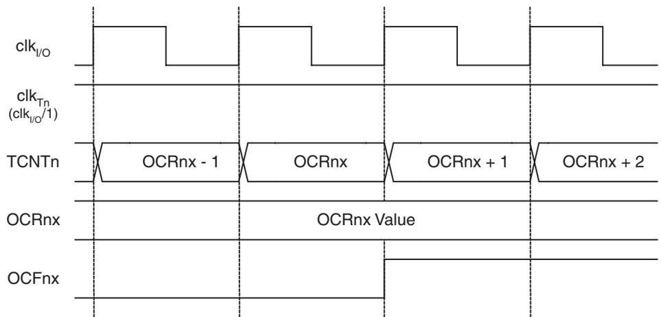
Figure 58 shows the same timing data, but with the prescaler enabled.
