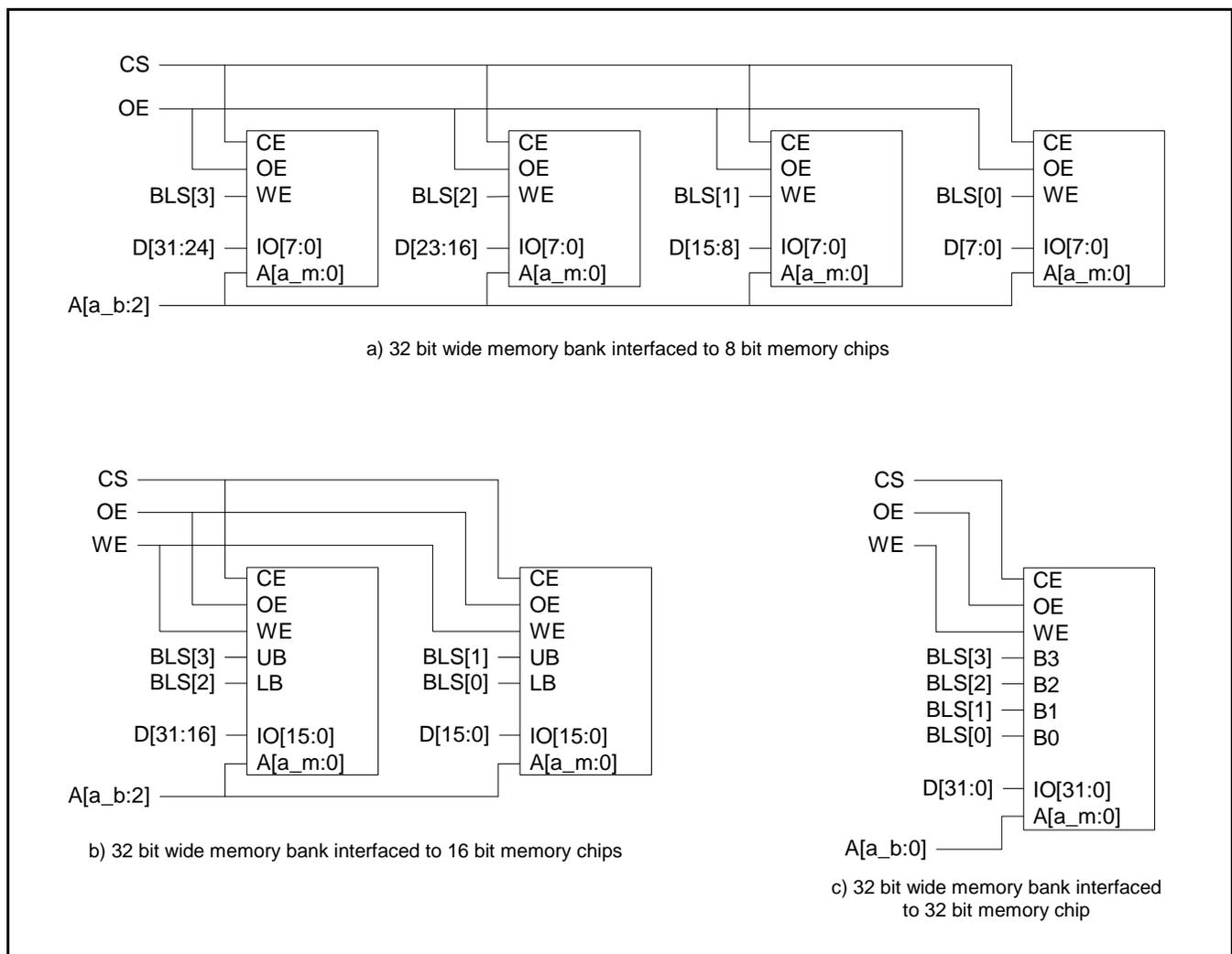
Figure 7: 32 Bit Bank External Memory Interfaces
