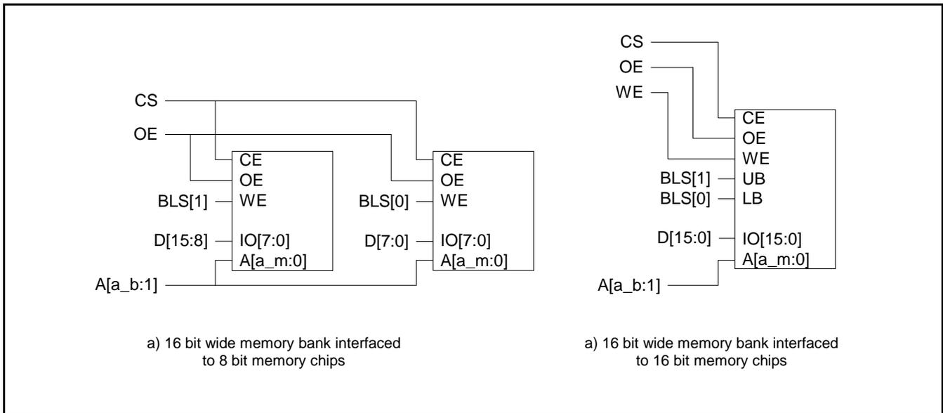
Figure 8: 16 Bit Bank External Memory Interfaces
