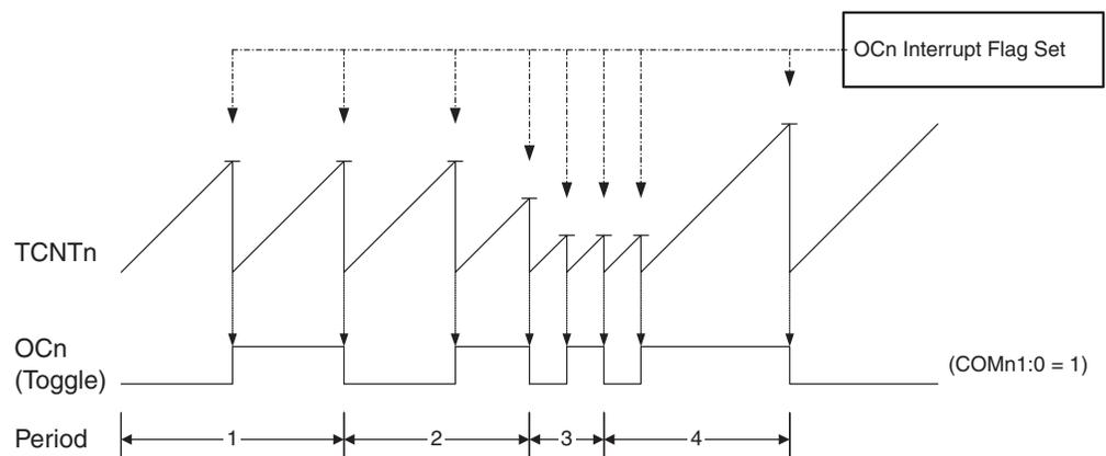
An interrupt can be generated each time the counter value reaches the TOP value by using the OCF2 Flag. If the interrupt is enabled, the interrupt handler routine can be used for updating the TOP value. However, changing the TOP to a value close to BOTTOM when the counter is running with none or a low prescaler value must be done with
