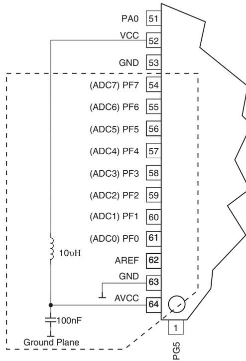
**Figure 122.** ADC Power Connections, ATmega640/1280/2560
