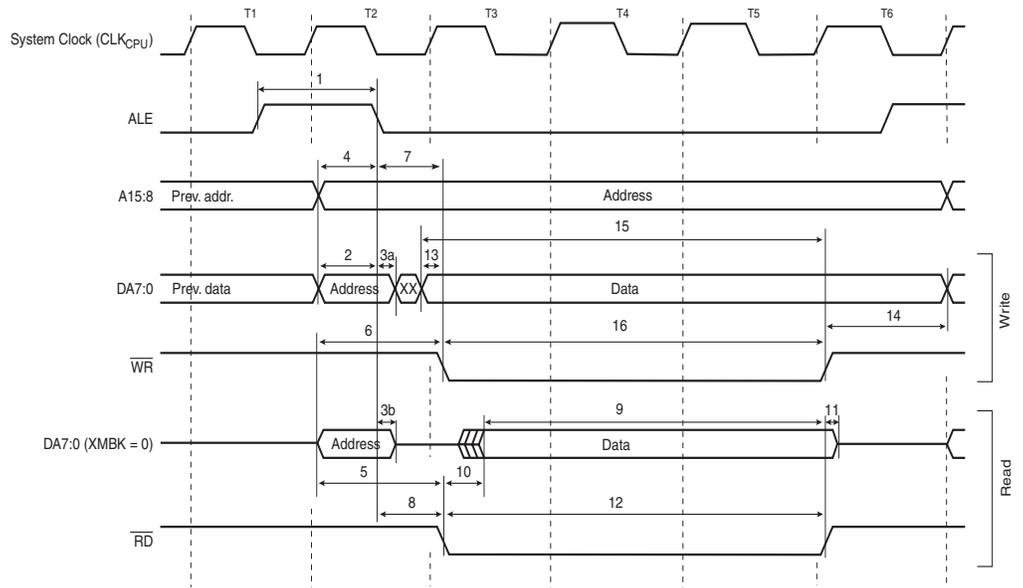
**Figure 166. External Memory Timing (SRWn1 = 1, SRWn0 = 1)<sup>0</sup>**
