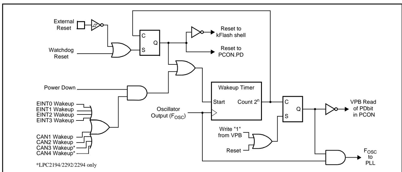
Figure 16: Reset Block Diagram including Wakeup Timer
