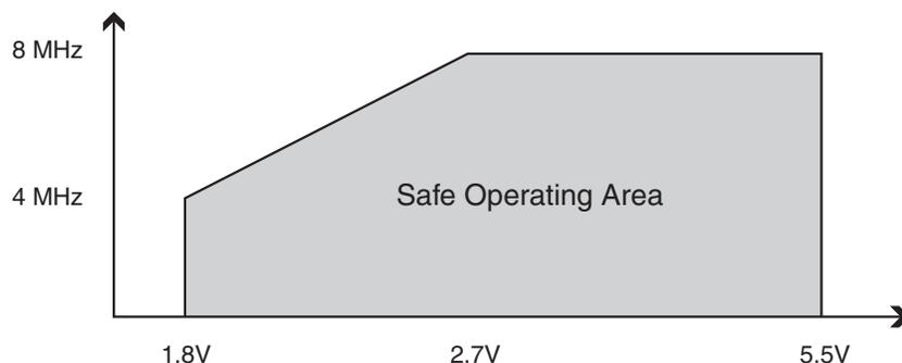
**Figure 157.** Maximum Frequency vs.  $V_{CC}$  when only using No-Read-While-Write Section<sup>(1)</sup>, ATmega2560V/ATmega2561V
