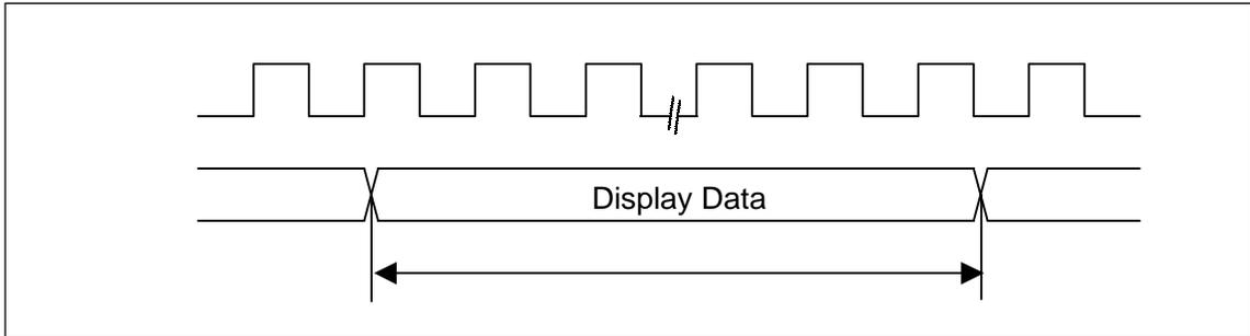
Figure 4-5 Basic read cycle of display memory
