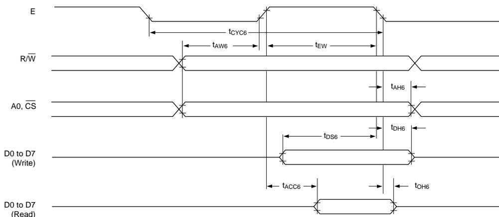
**Note:**  $t_{CYC6}$  indicates the interval during which CS is LOW and E is HIGH.
