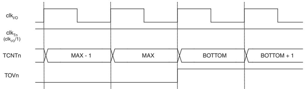
Figure 45 shows the same timing data, but with the prescaler enabled.
