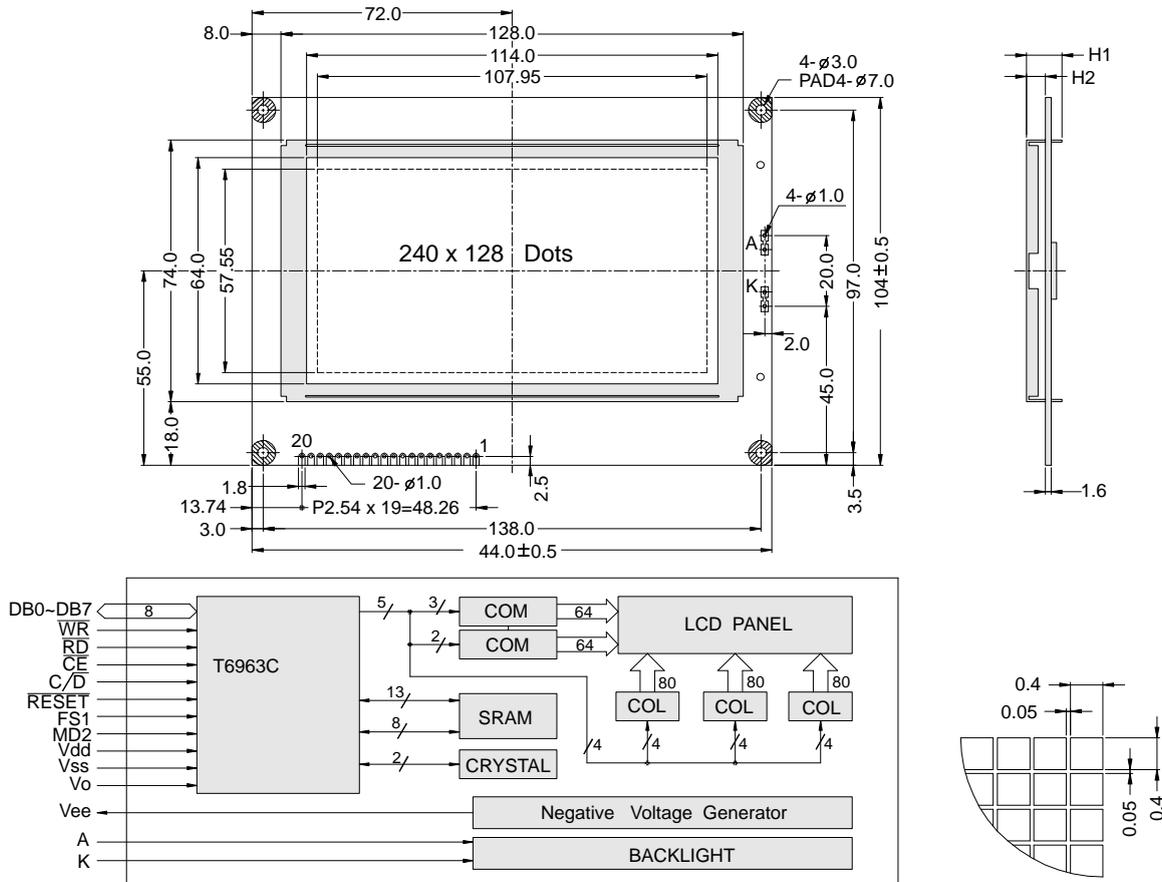
The tolerance unless classified  $\pm 0.3\text{mm}$
