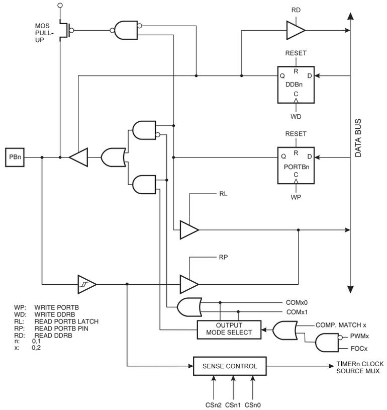
**Figure 57. Port B Schematic Diagram (Pin PB2)**
