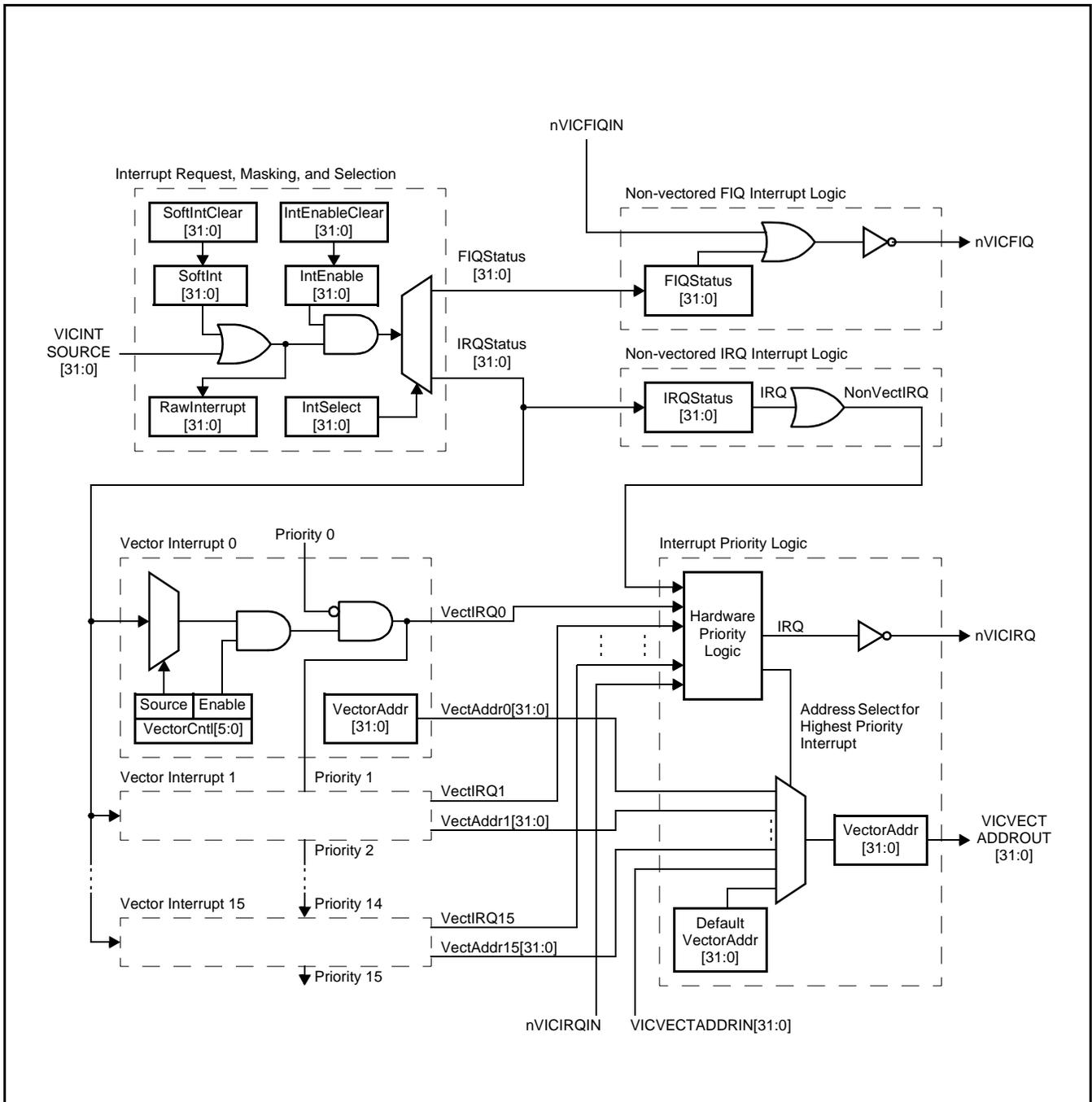
Figure 19: Block Diagram of the Vectored Interrupt Controller
