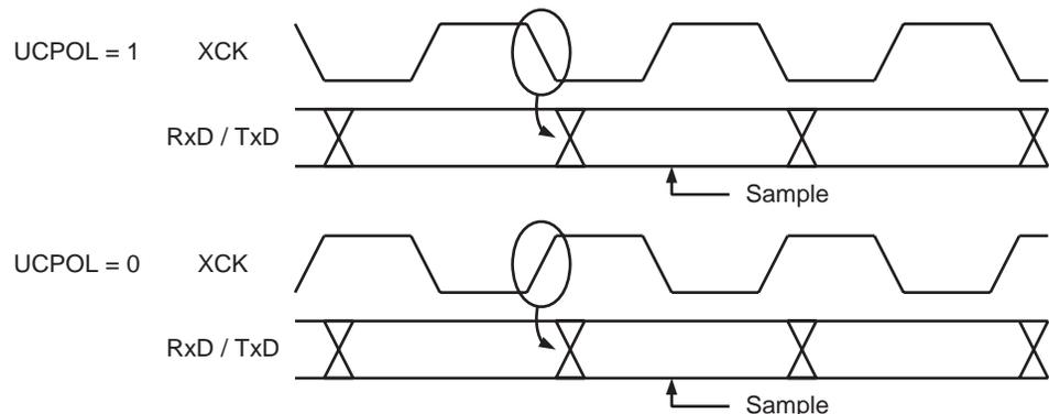
The UCPOLn bit UCRSC selects which XCKn clock edge is used for data sampling and which is used for data change. As Figure 84 shows, when UCPOLn is zero the data will be changed at rising XCKn edge and sampled at falling XCKn edge. If UCPOLn is set, the data will be changed at falling XCKn edge and sampled at rising XCKn edge.
