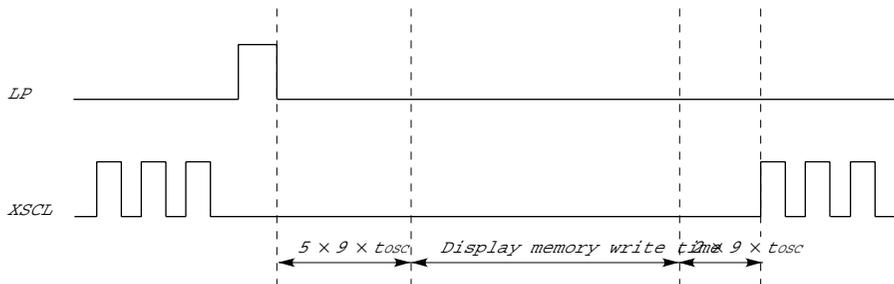
The allowable writing duration is since “ $5 \times 9 \times t_{osc}$ ” has elapsed ( $t_{osc} = 1/f_{osc}$ : a cycle of the oscillation frequency) from the positive going edge of LP up to  $\{(TCR) - (C/R) - 7\} \times 9 \times t_{osc}$ .
