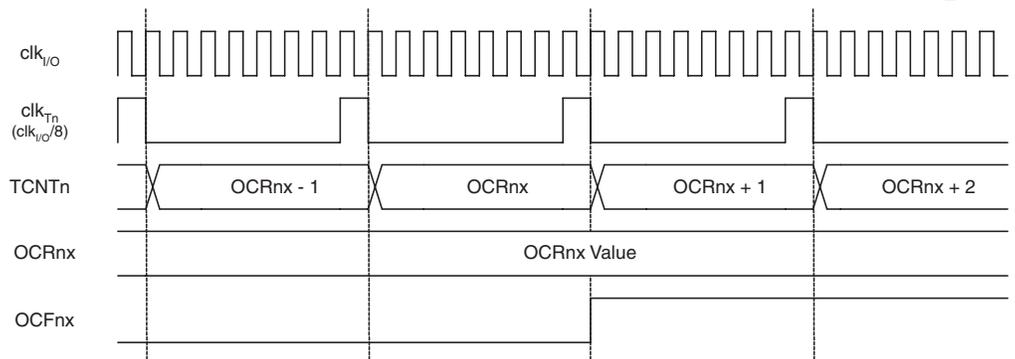
Figure 47 shows the setting of OCF0A and the clearing of TCNT0 in CTC mode and fast PWM mode where OCR0A is TOP.
