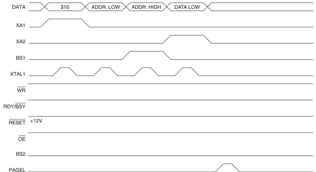
**Figure 77.** Programming the Flash Waveforms (Continued)
