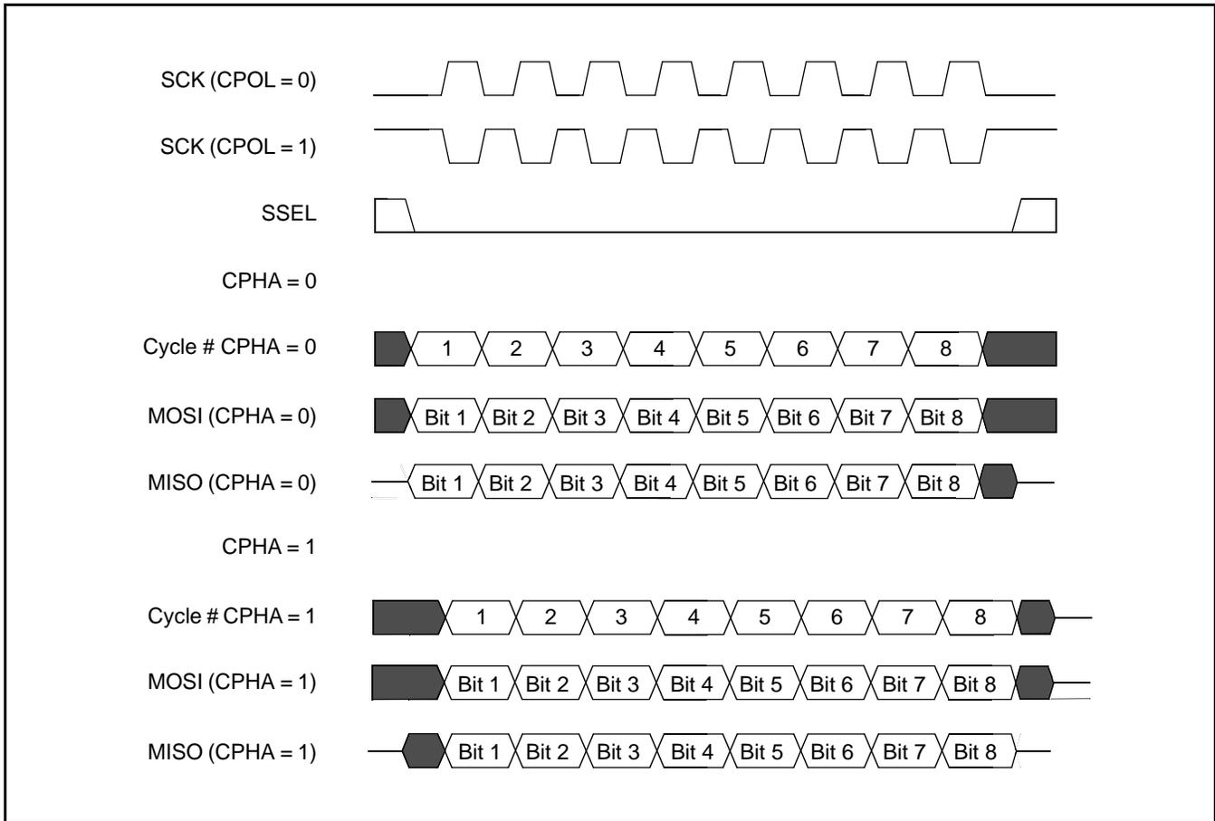
**Figure 33: SPI Data Transfer Format (CPHA = 0 and CPHA = 1)**
