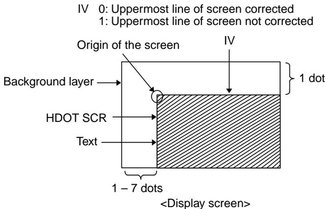
Figure 3-1 Combination of IV and HDOT SCR
