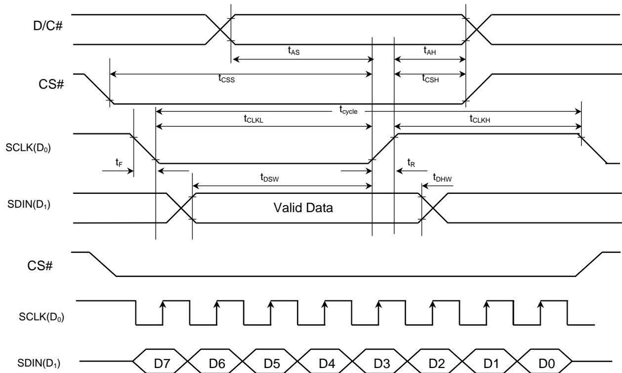
**Figure 12 - Serial Interface Characteristics**
