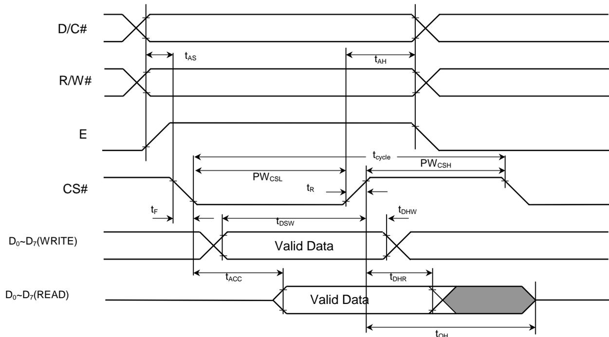
**Figure 10 - 6800-series MPU Parallel Interface Characteristics**
