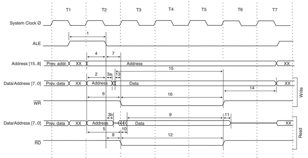
Note: 1. The ALE pulse in the last period (T4 - T7) is only present if the next instruction accesses the RAM (internal or external). The data and address will only change in T4 - T7 if ALE is present (the next instruction accesses the RAM).
