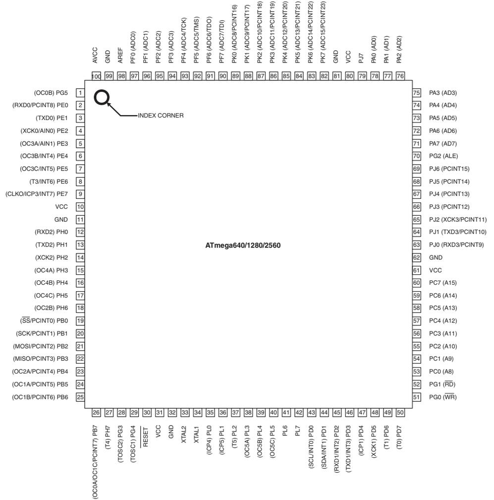
**Figure 2.** CBGA-pinout ATmega640/1280/2560
