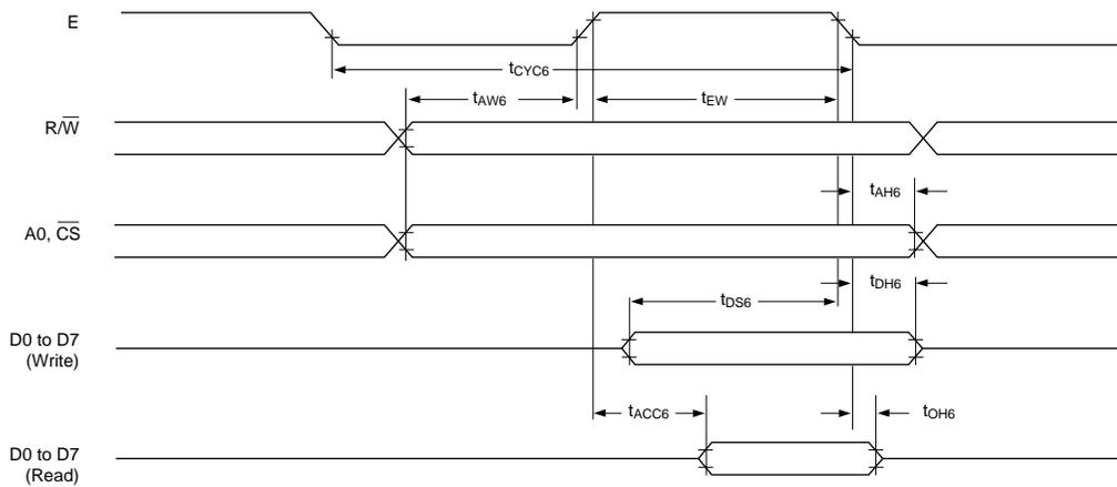
**Note:** t<sub>CYC6</sub> indicates the interval during which CS is LOW and E is HIGH.
