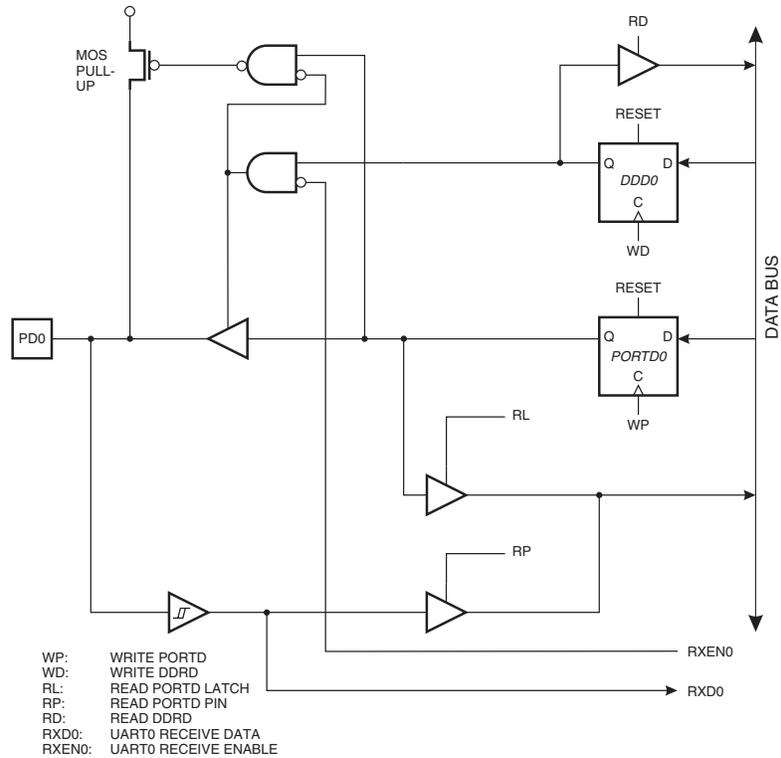
**Figure 65.** Port D Schematic Diagram (Pin PD1)
