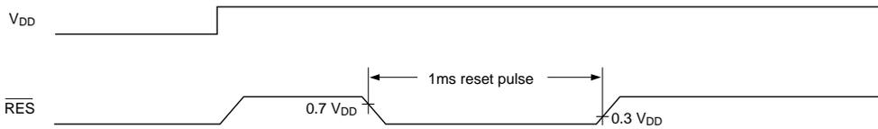
Figure 56. Reset timing
