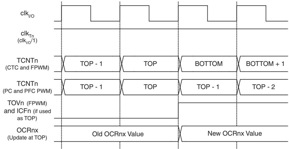
Figure 60 shows the same timing data, but with the prescaler enabled.
