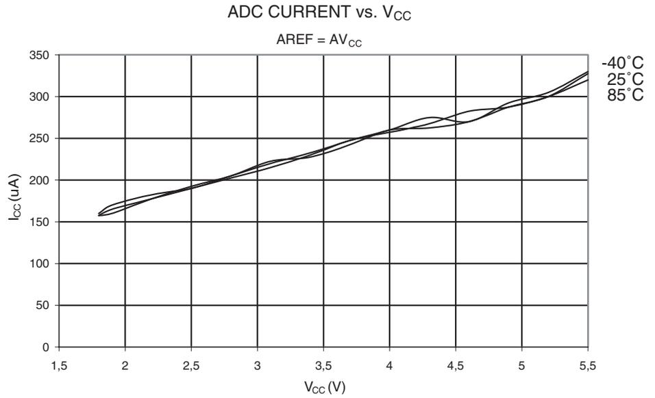
**Figure 208.**  $A_{REF}$  External Reference Current vs.  $V_{CC}$
