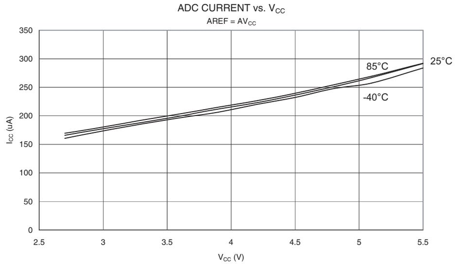
**Figure 208.** Aref External Reference Current vs.  $V_{CC}$
