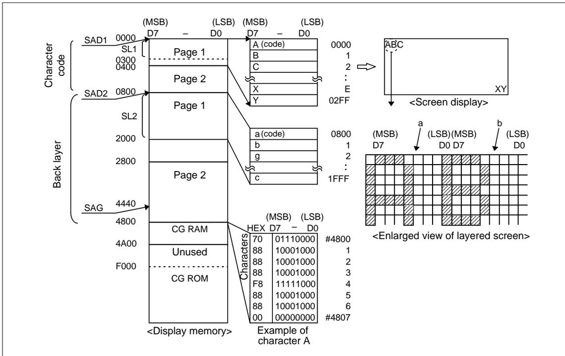
Figure 4-9 Example of display memory mapping
