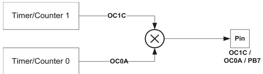
When the modulator is enabled, the two output compare channels are modulated together as shown in the block diagram (Figure 63).
