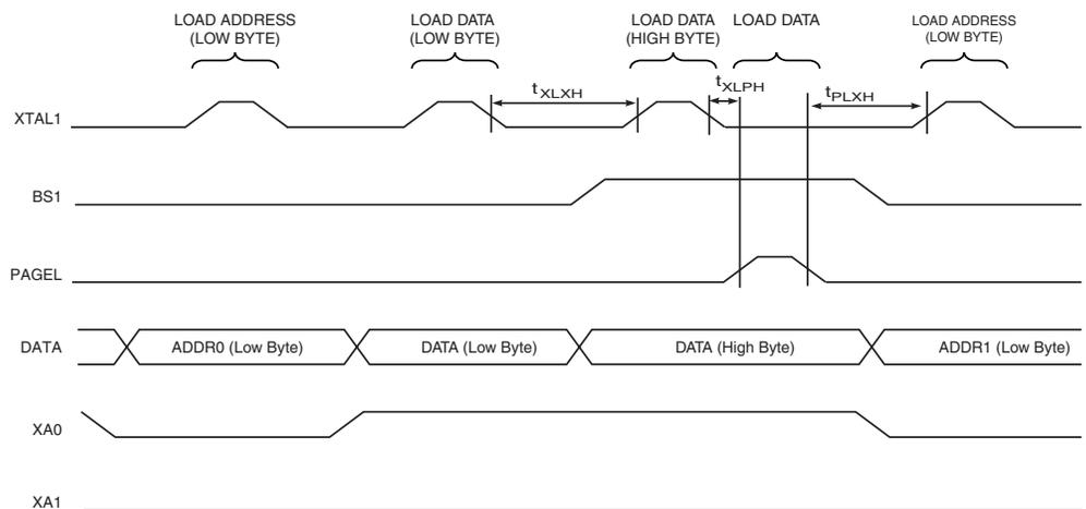
Note: 1. The timing requirements shown in Figure 144 (i.e.,  $t_{DVXH}$ ,  $t_{XHL}$ , and  $t_{XLDX}$ ) also apply to loading operation.
