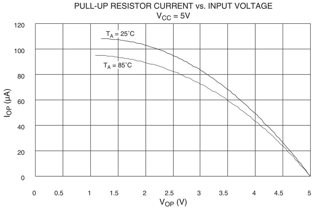
**Figure 92.** Pull-up Resistor Current vs. Input Voltage
