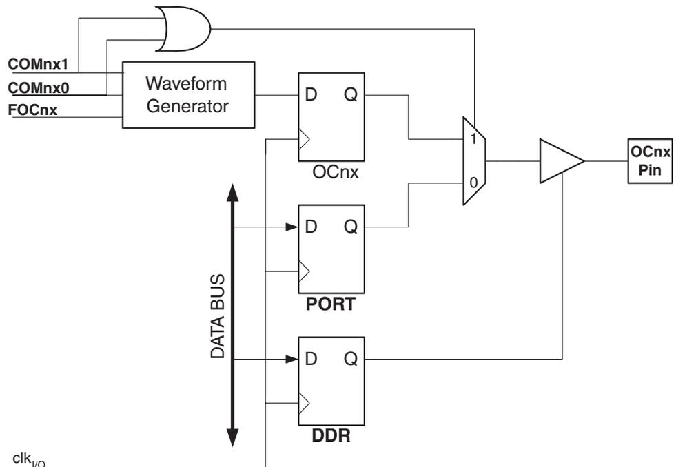
The general I/O port function is overridden by the Output Compare (OC2x) from the Waveform Generator if either of the COM2x1:0 bits are set. However, the OC2x pin direction (input or output) is still controlled by the Data Direction Register (DDR) for the
