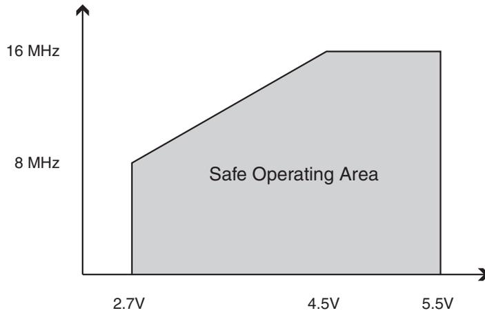
**Figure 159.** Maximum Frequency vs.  $V_{CC}$ , ATmega2560/ATmega2561
