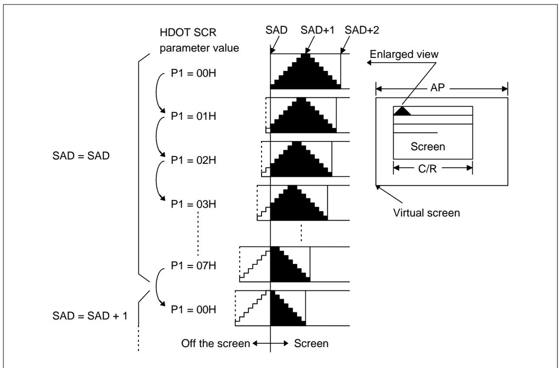
Figure 4-10 Example of using HDOT SCR ([FX] = 8)
