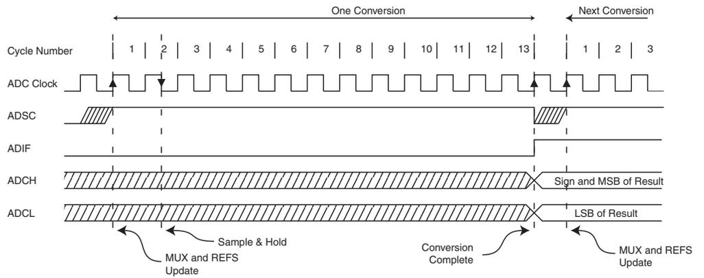
**Figure 118. ADC Timing Diagram, Auto Triggered Conversion**
