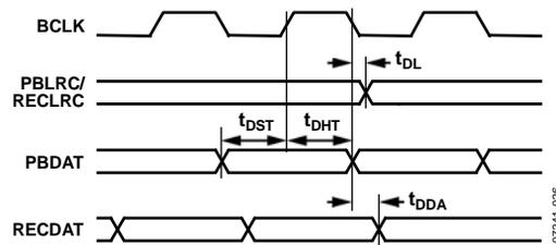
Figure 4. Digital Audio Interface Master Mode Timing
