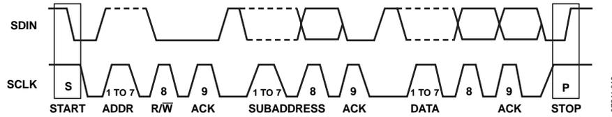
Figure 28. 2-Wire I<sup>2</sup>C Generalized Clocking Diagram
