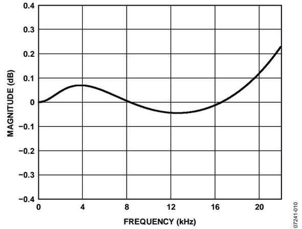
Figure 14. De-Emphasis Error, Audio Sampling Rate = 44.1 kHz
