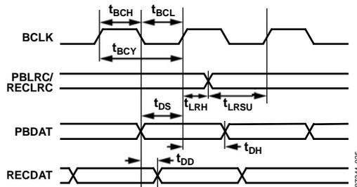
Figure 3. Digital Audio Interface Slave Mode Timing
