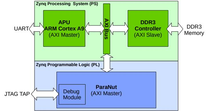
Fig. 8: Block diagram of the *ParaNut/RISC-V* system
