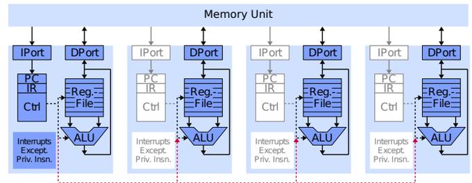
Fig. 2: *ParaNutm* processor operating in *linked mode*
