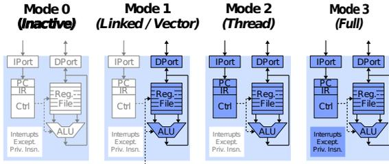
Fig. 5: Modes of a *ParaNut* core
