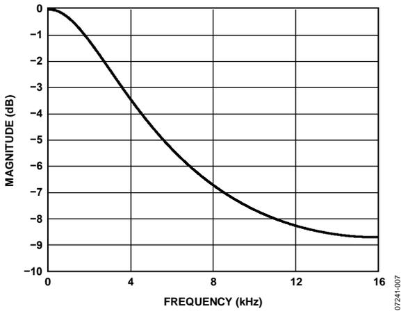
Figure 11. De-Emphasis Frequency Response, Audio Sampling Rate = 32 kHz
