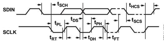
Figure 2. I<sup>2</sup>C Timing
