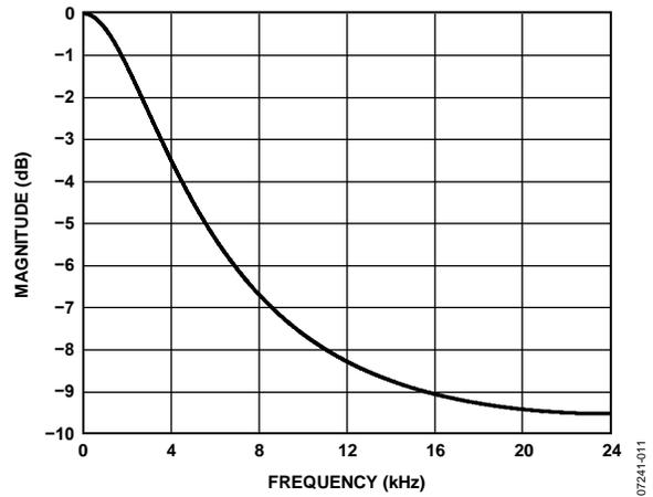
Figure 15. De-Emphasis Frequency Response, Audio Sampling Rate = 48 kHz
