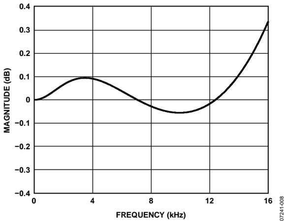
Figure 12. De-Emphasis Error, Audio Sampling Rate = 32 kHz
