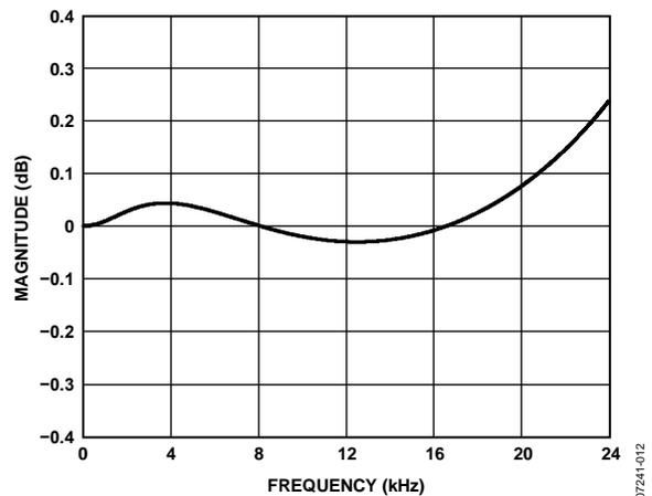
Figure 16. De-Emphasis Error, Audio Sampling Rate = 48 kHz
