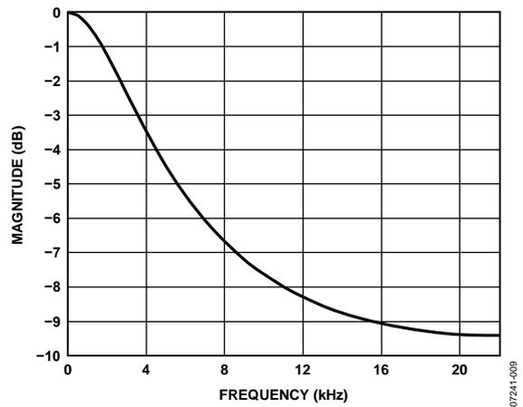
Figure 13. De-Emphasis Frequency Response, Audio Sampling Rate = 44.1 kHz
