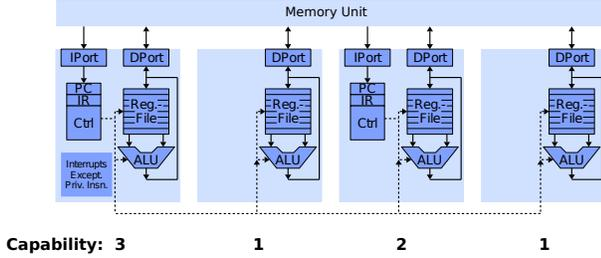
Fig. 6: Example of a *ParaNut* instantiation with cores of different capabilities
