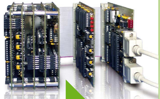
figure [4]: Smallest possible MyCPU computer system
