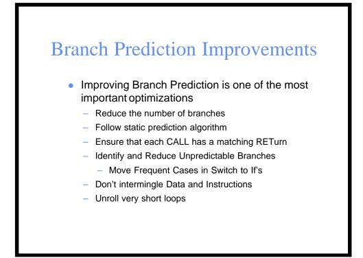
The mixing of data in the instruction stream causes the front end of the machine to be sent off on a fruitless mission. Decoder bandwidth is consumed and in some cases data may be speculatively executed. This is not damaging in the sense that the external world is aware of this but it is damaging in the sense that BTB values may be corrupted and ICache locations are polluted. There is also potential for CALL /RETurn synchronization to be lost unnecessarily.
