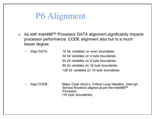
Data alignment is very important on P6. Misaligned data accesses are completed at retirement and as such are expensive. All data should be aligned on the data types natural boundary.
