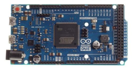
Figure 15: Arduino Due
