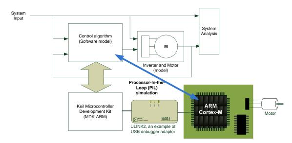
Figure 10: Running example control application in Simulink with Processor-in-the-Loop (PIL)
