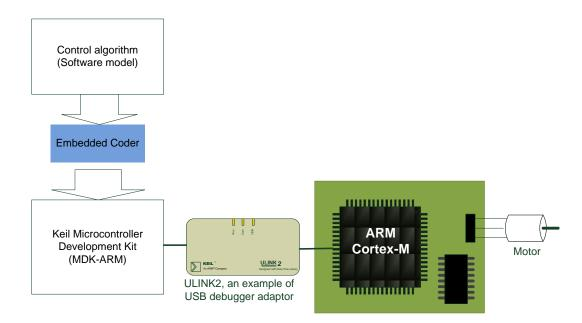
Figure 11: Transfer of control application developed in Simulink to hardware platform
