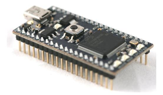
Figure 17:A mbed board with NXP LPC1768 microcontroller
