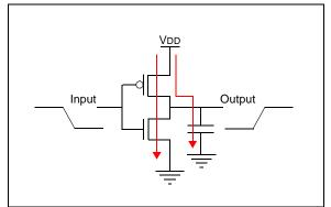
This inverter will consume little to no power when the input is at VDD or VSS. However, when the signal switches from VDD to VSS, there is a transition period where the PMOS and NMOS will both be biased in the linear region, allowing current to flow from VDD to ground. Also note, in a real system there is some amount of load capacitance on the output bus. There is additional current consumption associated with the charging and discharging of this bus capacitance when the logic level changes.
