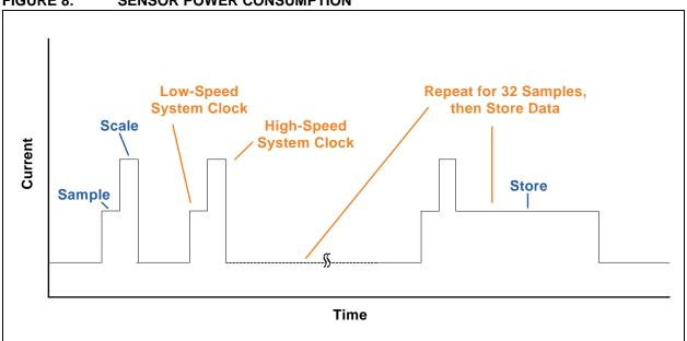
FIGURE 8: SENSOR POWER CONSUMPTION
