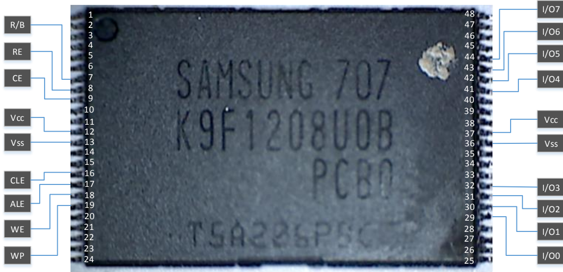
Figure 5 Important NAND Flash memory pins and names
