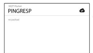
When the broker receives a PINGREQ packet, the broker must reply with a PINGRESP packet to show the client that it is still available. The PINGRESP packet also does not contain a payload.
