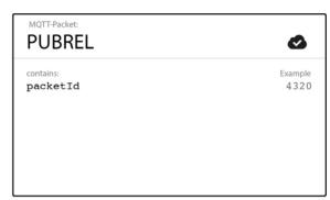
Once the sender receives a PUBREC packet from the receiver, the sender can safely discard the initial PUBLISH packet. The sender stores the PUBREC packet from the receiver and responds with a PUBREL packet.
