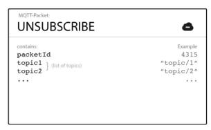
**Packet Identifier**: The packet identifier uniquely identifies a message as it flows between the client and broker. The client library and/or the broker is responsible for setting this internal MQTT identifier.
