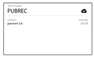
When a receiver gets a QoS 2 PUBLISH packet from a sender, it processes the publish message accordingly and replies to the sender with a PUBREC packet that acknowledges the PUBLISH packet. If the sender does not get a PUBREC packet from the receiver, it sends the PUBLISH packet again with a duplicate (DUP) flag until it receives an acknowledgement.
