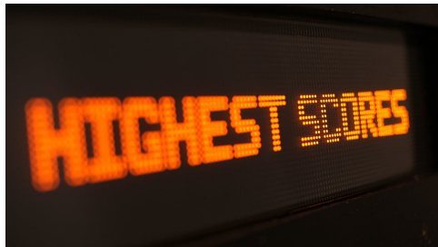
A monochrome dot-matrix display
