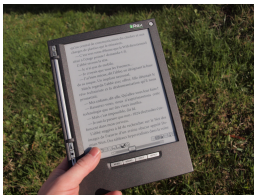
An e-reader with an EPD display
