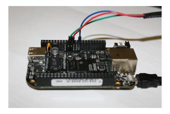
Once the USB to Serial connector is plugged in, a new serial port should appear: /dev/ttyUSB0. You can also see this device appear by looking at the output of dmesg.
