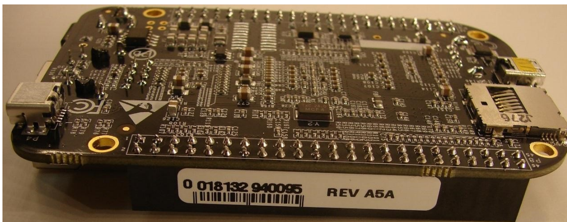
Figure 78. Third Phase Serial Number and Revision Location
