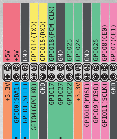
Raspberry Pi GPIO connector (P1) pinout
